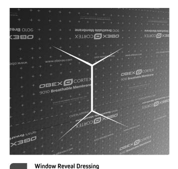
Cut the Membrane from the center of the window
