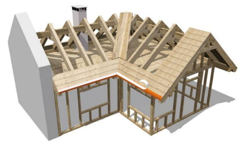
Apply a strip of OBEX CORTEX Double-Sided Tape along the eaves line. Do not remove the release liner from the double-sided tape yet.
