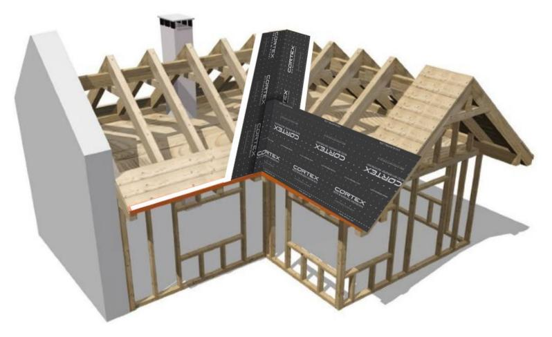
Starting along the eaves line with the membrane lapping over the verge, install the membrane along the roof and extend over any valleys and onto the adjacent pitch. Tack the membrane in place as you go. The overlap in the verge will be covered by the soffit and fascia detail.
