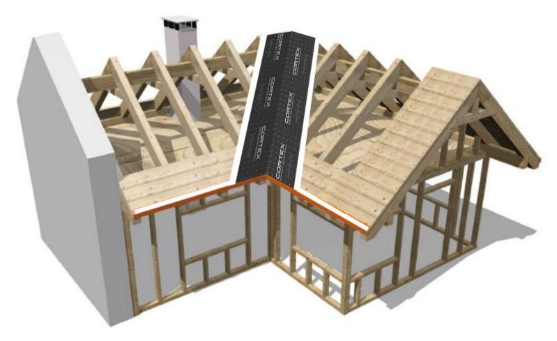
Install the OBEX CORTEX 9010 Breathable Membrane down any roof valleys. Tack the membrane in place, and fold back along the eaves line and remove the release liner from the double-sided tape. Bond the membrane onto the double-sided tape.
