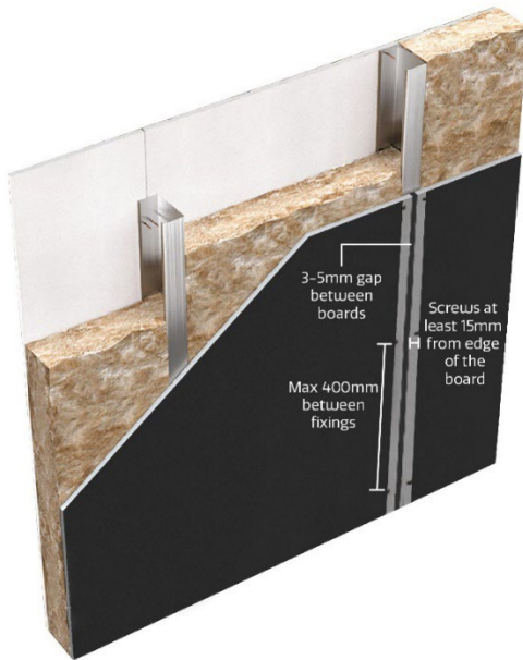
Diagram 1 - Typical detail of fixing layout
