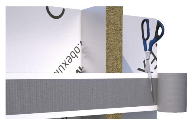
Cut the membrane to length with membrane shears.
