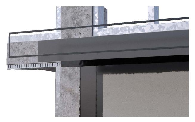
Repeat steps 2-5 for the head of the board infill section. Ensure an overlap of at least 100mm onto the Interface Sealing Membrane on the sides. A wider width of membrane may be required to allow for the deflection head gap.
