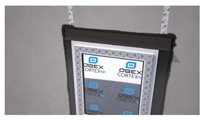
Bond the O2OOFR Membrane to the frame first, and then bond back to the substrate. Ensure the membrane is applied flat, without creases, and tension free.
