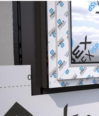
Cut around any penetrations, ensuring that the Breather Membrane overlaps the ISM (Interface Sealing Membrane). Ensure to cut 30-40mm from the penetration so that there is room to apply tape at a later stage.
