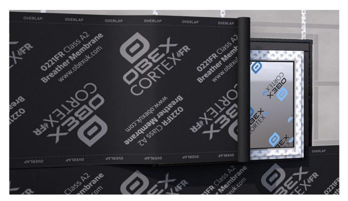
Repeat steps 1-5 until the section of the wall is covered. Horizontal laps should be 100 mm and vertical laps 150 mm. Vertical laps should also be staggered where possible. Corner overlaps should be at least 300 mm.
