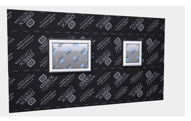
This is how a correctly overlapped wall should look. Note upper layers are installed over lower layers.
