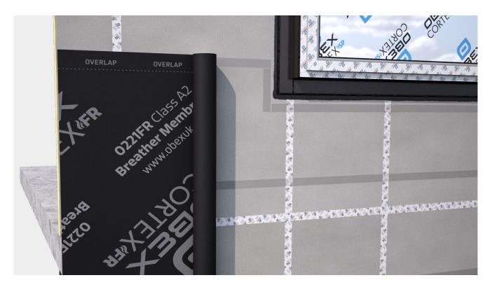
You're now ready to apply the breather membrane. Place the roll into position to cover the strips of double-sided tape and start rolling the membrane over the tape.
