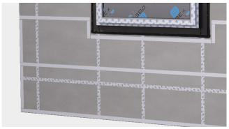
Start by applying the OBEX CORTEX 0824FR Double-Sided Tape; 3 strips to cover the width of the membrane (allowance for a 100 mm horizontal lap should be made). After this, apply tape to ensure all edges of the membrane will be adhered e.g. where the membrane is cut around windows and other penetrations.
