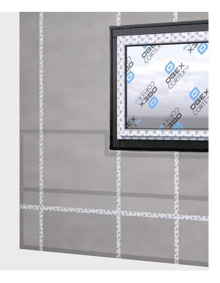
Once the previous step is complete, peel off the release liner from the OBEX CORTEX 0824FR Double-Sided Tape. Some may prefer to remove the release liner as they adhere the membrane.
