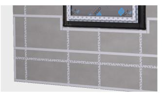
Start by applying the OBEX CORTEX 0824FR Double-Sided Tape; 3 strips to cover the width of the membrane (allowance for a 100 mm horizontal lap should be made). After this, apply tape to ensure all edges of the membrane will be adhered e.g. where the membrane is cut around windows and other penetrations.
