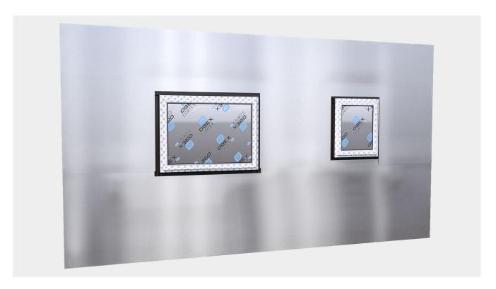
This is how a correctly overlapped wall should look. Note upper layers are installed over lower layers and the reflective face of the membrane facing out from the building.
