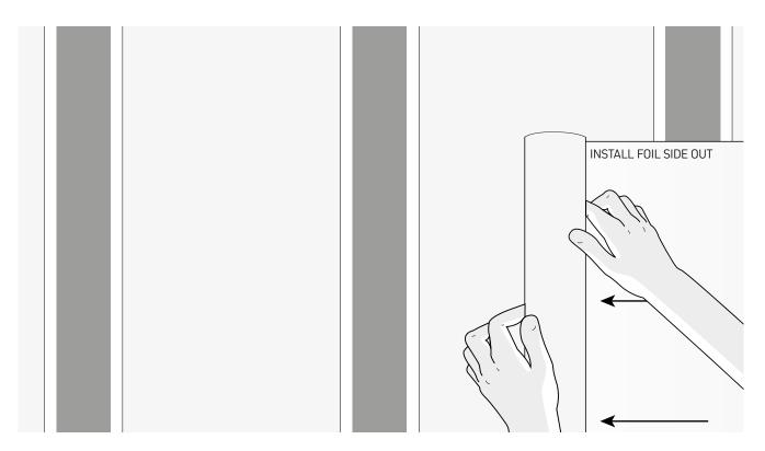
Apply the vapour control layer over the double-sided tape in horizontal strips starting from the base. It is recommended that the next layer should overlap the previous layer by 50mm. The membrane MUST be installed with the silver foil side visible to the installer.
