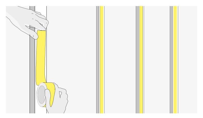
Start by applying the OBEX CORTEX 0824FR Double-Sided Tape to the vertical studs at one end of the application and repeat this process on every vertical stud. Consider where fixings may penetrate the vapour control layer and ensure that double-sided tape is present at these locations.
