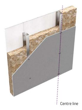
Offer up the board into position, ensuring the edges of the board are just shy of the centre line of the framing member to leave the recommended 3-5mm gap.
