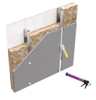
For EI60 compliance, all board joints and fixing heads should be sealed using OBEX CORTEX 0280 Board Sealant.
