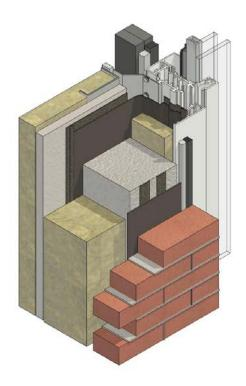
The perimeter of the framing sections of windows, doors, and other openings shall be sealed from the board to the RC or steel structure using a suitable ISM (Interface Sealing Membrane) from the OBEX CORTEX range. For relevant buildings, membranes used as part of the external wall construction must achieve a minimum of B-s3,d0 according to EN13501-1.
