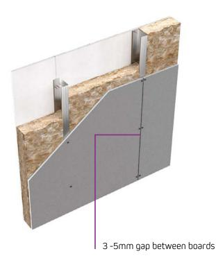
Horizontal and vertical joints should be staggered. When fixing adjacent boards, leave a gap of 3-5mm between the boards to ensure correct installation. Board joints should not coincide at the corners of any windows, doors, or openings.
