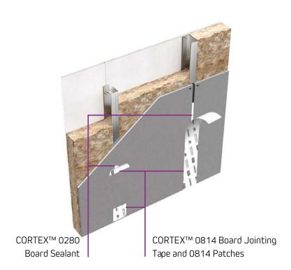
Additional weather performance can be achieved by applying the OBEX CORTEX 0814 tape over the joints sealed with 0280 sealant. Where El60 is not required, OBEX CORTEX 0814 Board Jointing Tape & Patches may be used to seal the joints and fixing heads.
