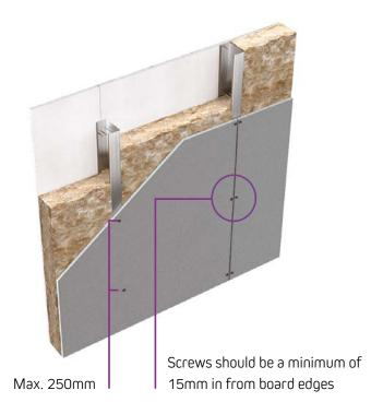
0290FR Screws should be used to fix the board to the support framing (for steel up to 3mm thick). Screws should be a minimum of 15mm in from the board edges, spaced at a maximum of 250mm centres and must not be overtightened. (Screws should penetrate a minimum of 10mm through steel and 25mm into timber). The board should not be fixed into expansion head track.
