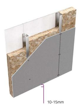
Boards should sit 10-15mm above any deck or slab to avoid standing water. An offcut of board can be placed underneath the board to ensure this is achieved.
