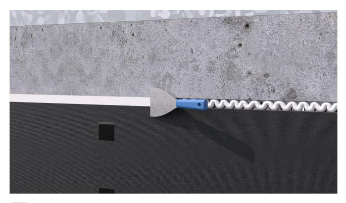
Fill expansion gap at the head flush with OBEX CORTEX 0280FR Board Sealant.
