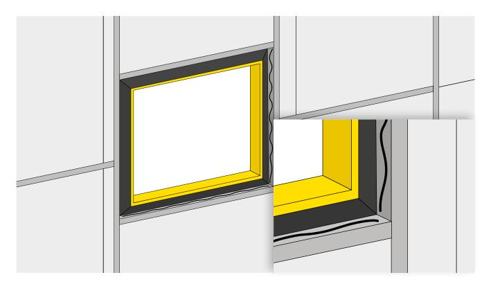
Apply paste to the inside of the window reveal on all sides. Also apply paste to the membrane overlaps.
