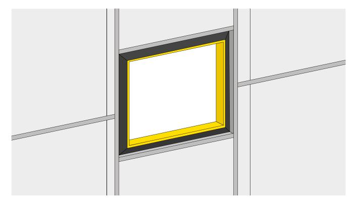
Fold the membrane away from the sides of the reveal and temporarily secure to enable the application of paste onto the sides of the window reveal.
