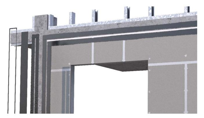
Repeat steps 2-5 for the sides of the board infill section. Ensure an overlap of at least 100mm onto the Interface Sealing Membrane on the base.
