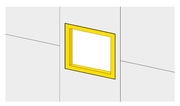
Insert The Frame Within The Opening & Fix Within The Reveal According To The Manufacturers Instructions
