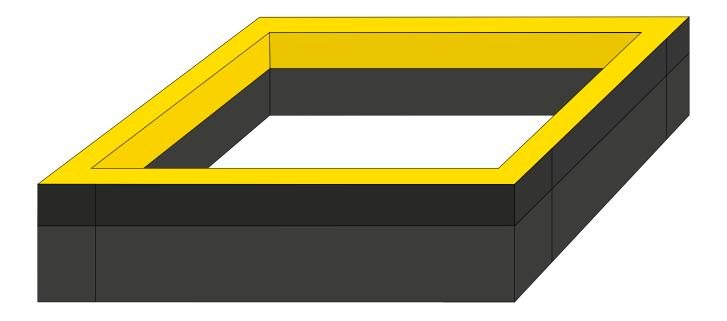
Continue Steps 6-9 To Apply Membrane To The Bottom Of The Window Frame
