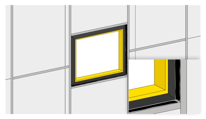
Spread the paste out using a spreader ensuring there are no gaps to ensure a complete seal.
