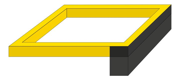
Fold Both Membrane Flaps On Each Side And Ensure The Mebrane Is Firmly Bonded Onto The Paste By Bedding-In With A Silicone Roller.
