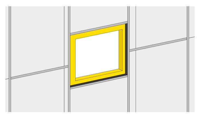
Use a roller to adhere the membrane to the opening and then cap the edges off with paste. Also Remember To Cap Off The Membrane Overlap Joints.
