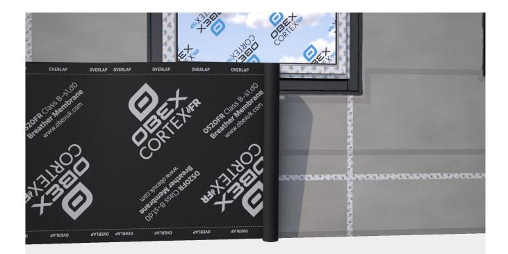
Where possible, the membrane should be continuous so any window/door openings or penetrations should be cut out during application, or it can be applied over the top and cut out afterwards.
