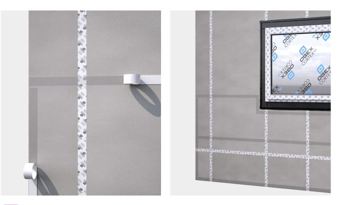
Once the previous step is complete, peel off the release liner from the OBEX CORTEX 0824FR Double-Sided Tape. Some may prefer to remove the release liner as they adhere the membrane.
