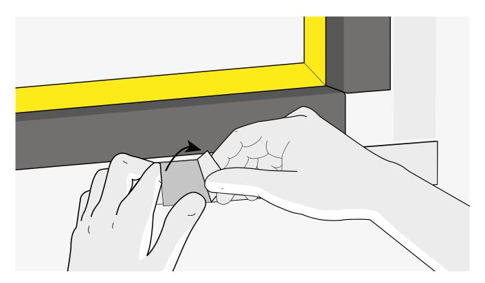
Once the previous step is complete, peel off the release liner from the OBEX CORTEX 0824FR Double-Sided Tape. Some may prefer to remove the release liner as they adhere the membrane.
