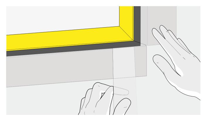
Where possible, the membrane should be continuous so any penetrations should be cut out during application, or it can be applied over the top and cut out afterwards. Horizontal laps should be 100 mm and vertical laps 150 mm. Vertical laps should also be staggered where possible. Corner overlaps should be at least 300 mm.
