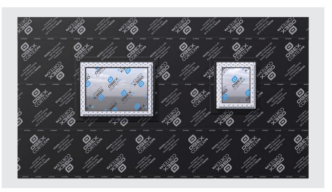
Make such that each layer of membrane overlaps the one below by 100mm.
