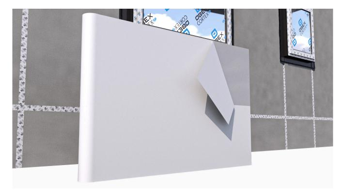
Peel back a section of the top release liner and apply the top corner of the membrane onto the substrate at the desired position. Start from the bottom and work upwards, ensuring that upper layers lap over lower layers.
