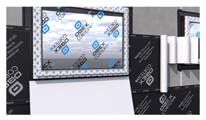
Fold the cutout down and continue to remove the upper section of the release liner, bonding the membrane to the wall.
