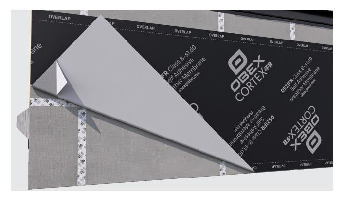
Now peel away the lower section of the release liner and affix the membrane to the substrate as before.
