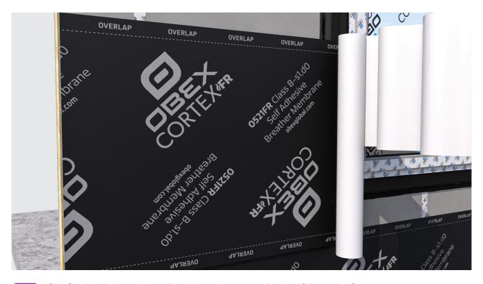
If the façade includes windows, adhere the membrane up to the edge of the window frame.
