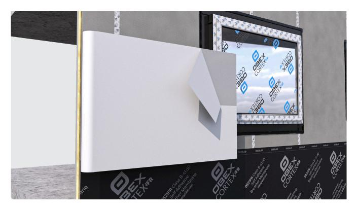
For additional horizontal layers, repeat the process, ensuring that each layer overlaps the one below by a minimum of 100mm.
