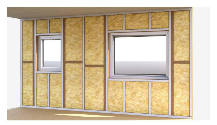
$Apply\ OBEX\ CORTEX\ 0850\ Double-Sided\ Tape\ to\ the\ studs\ and\ head\ track,\ considering\ where\ fixings\ may\ penetrate\ the\ vapour\ control\ layer\ and\ ensure\ that\ double-sided\ tape\ is\ present\ at\ these\ locations.$
