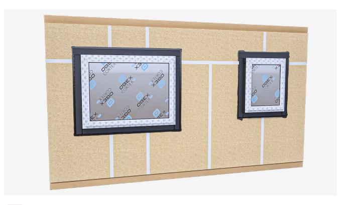
Install the timber studs and sheathing board as per manufactures instructions. Ensure board joints are sealed. Ensure EPDM has been installed correctly around windows & protrusions.
