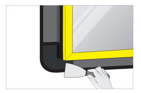
Tool off the paste adhesive with a spreader to ensure no open edges.
