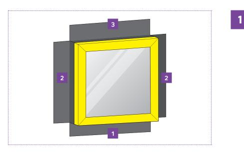
Cortex EPDM Membrane should be fitted in this order around the window: cill, jambs and then head.
