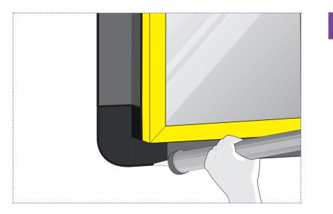
Corners can be sealed using Cortex 0901 External Corners. Apply a bead of Cortex Paste Adhesive around the perimeter of the membrane and any joints/laps.
