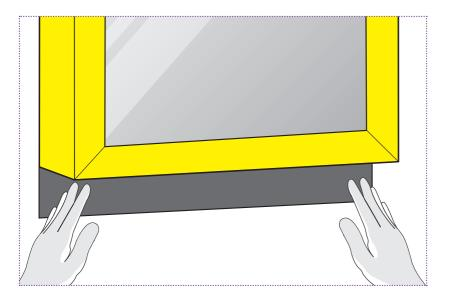
Now bond back to the substrate - ensuring the membrane is applied without creases.
