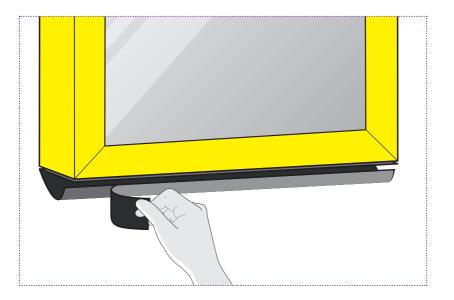
Remove the release liner from the other edge off the back of the EPDM Membrane.
