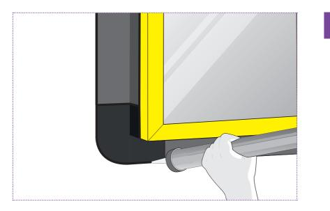
Corners can be sealed using Cortex 0901 External Corners. Apply a further bead of Cortex Paste Adhesive around the perimeter of the membrane and any joints/laps.
