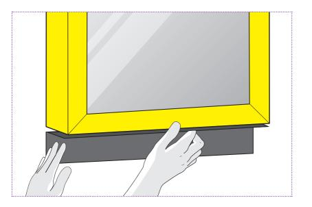
Bond the Cortex EPDM Membrane to the frame first, and then bond back to the substrate, ensuring the membrane is applied flat without creases.
