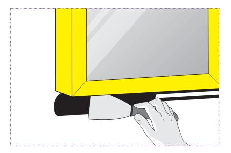
Spread out the paste adhesive using a paste adhesive spreader.
