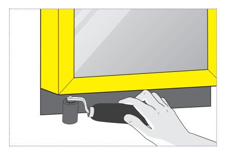
Roll firmly with a seam roller to ensure maximum bond strength on all surfaces.
