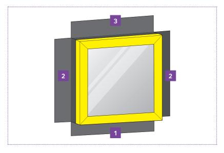
Cortex EPDM Membrane with Gasket should be fitted in this order around the window: cill, jambs and then head.
