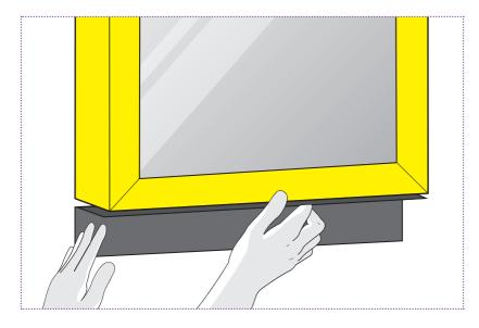
Clip the Cortex EPDM Membrane with Gasket into the carrier on the frame, and then bond back to the substrate, ensuring the membrane is applied flat and without creases.
