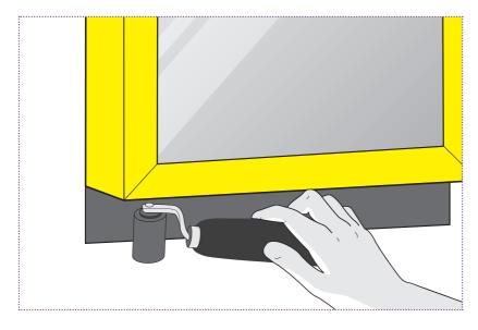
Roll firmly with a seam roller to ensure maximum bond strength to all surfaces.
