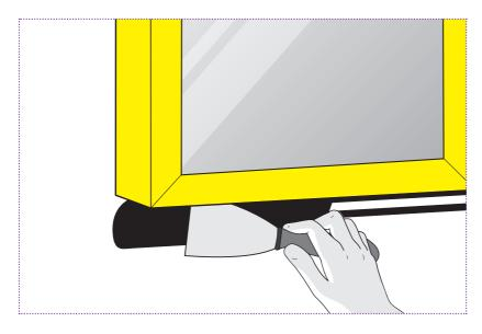
Spread out the paste adhesive using a paste adhesive spreader.
