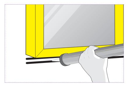
Apply a bead of Cortex Paste Adhesive into the gasket carrier using a paste adhesive gun. Then apply Cortex Paste Adhesive onto the substrate.
