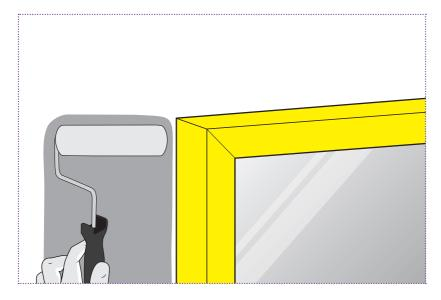
Ensure both substrates are clean, dry, and free from grease and oil prior to application. Porous surfaces may need to be primed using Cortex 0785 Primer.
