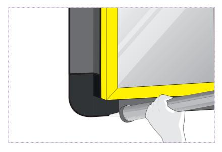
Corners can be sealed using Cortex 0901 External Corners. Apply a further bead of Cortex Paste Adhesive around the perimeter of the membrane and any joints/laps.
