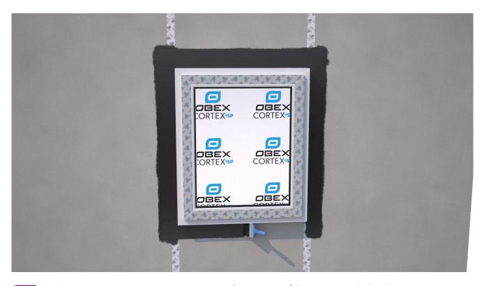
Apply OBEX CORTEX 0787FR Primer to porous surfaces. Ensure a full coverage over the bonding area. Porous surfaces include cement board, calcium silicate board, concrete etc.
