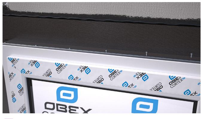
Locate the 0819 termination on top of the membrane. Ensure there is paste adhesive underneath the membrane to ensure the fixings are sealed. Using self-drilling screws or suitable screws for the glazing unit, fix the 0819FR termination bar through the pre-drilled holes.
