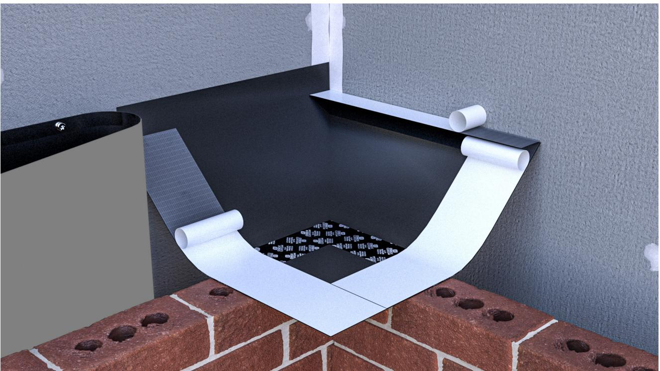
**10** Install the OBEX CORTEX 0243FR RapidTray Internal Corner. Start by removing the adhesive strip backing on the rear of the corner, then adhere to the wall. Then remove the adhesive strip backing on the front face of the corner. Remove one strip at a time for easier bonding and positioning.
